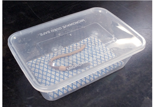
FIGURE 1. The earthworm egestion collection unit containing an adult Lumbricus terrestris . The portable containers (14 cm × 9 cm × 5 cm) were an economical and efficient means of immediately segregating large numbers of live earthworms in the field to collect gut contents. Photo: M. McTavish.
